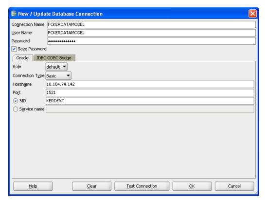
5. Click **Test Connection** and ensure it is successful. If connection fails, verify and repeat step 4
